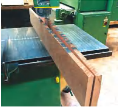
▲ Pic.1 The first step was to rough cut some timber. Ripping timber is always a bit of a tense moment, as you can never really tell how much the boards will spring back
